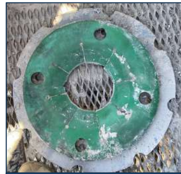
POLY ROD WIPER DISC AFTER 5 WEEKS
