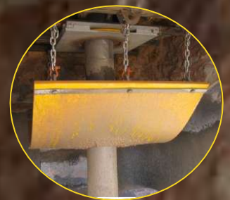
RUBBER ROD WIPER DISC AFTER 2 WEEKS
