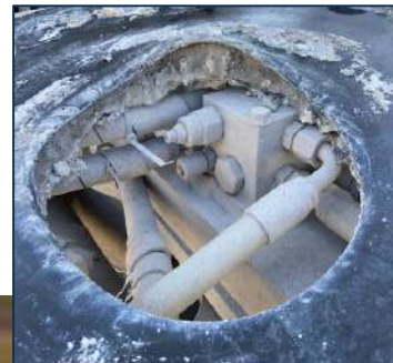
RUBBER ROD WIPER DISC AFTER 2 WEEKS
